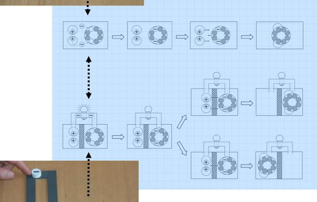
**Fuel cell**: Separating layer forces the electrons to detour via an conducting wire (=current)
